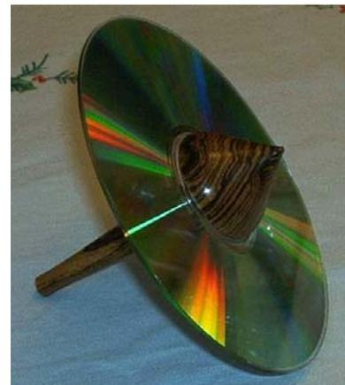
2. Shape the wood to the shape shown with the critical dimension being the diameter of the hole in the CD. The CD should slide over the handle of the top and rest flat on the base.
