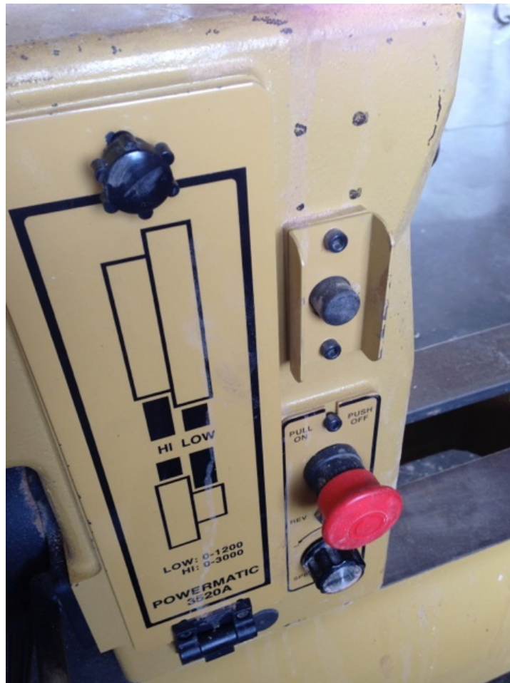
3520A Headstock front panel showing the four marked and center punched holes above the spindle lock button guard (upper right).
