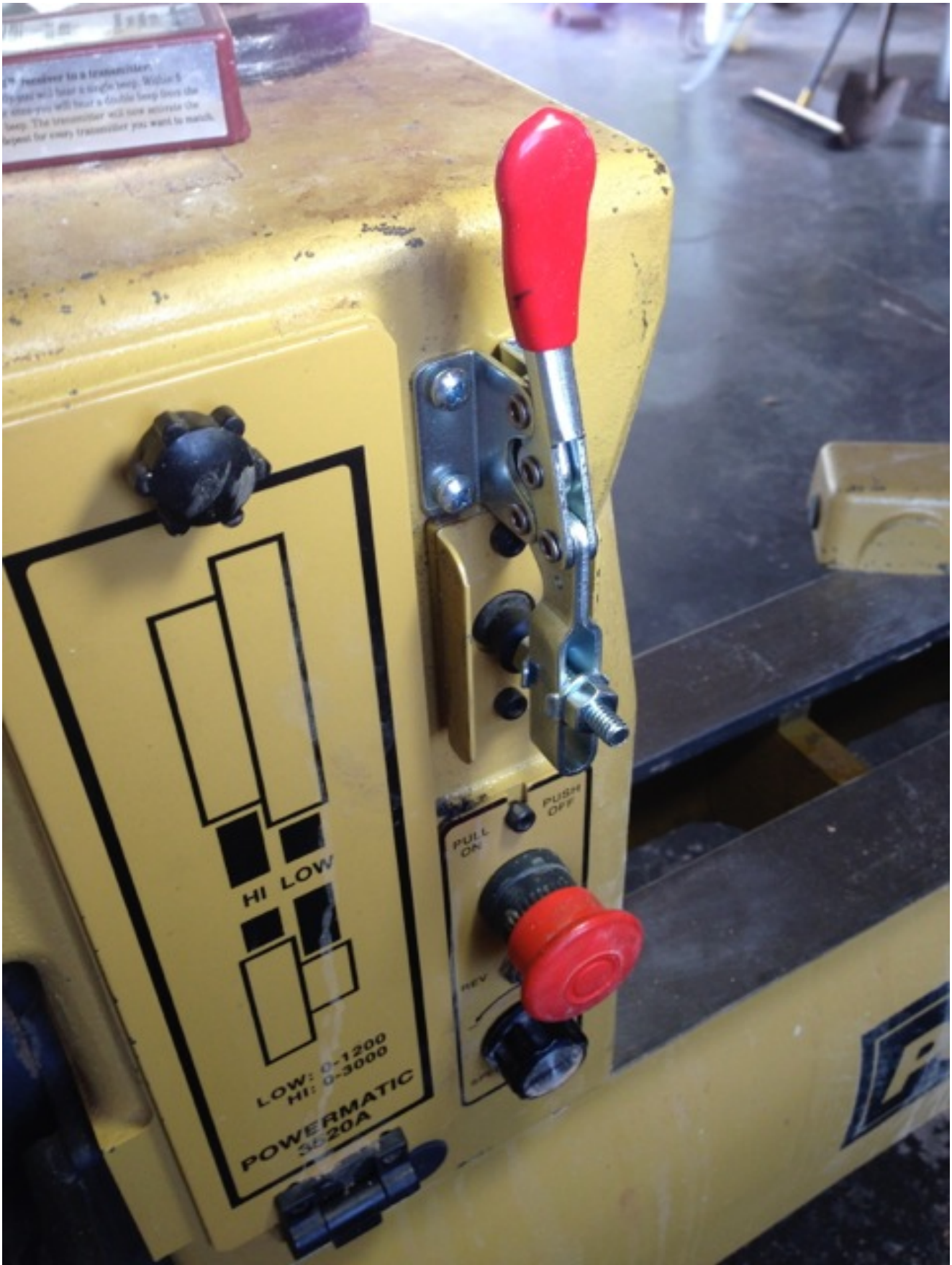
Toggle clamp installed. Clamp shown in the 'spindle is locked' position.
