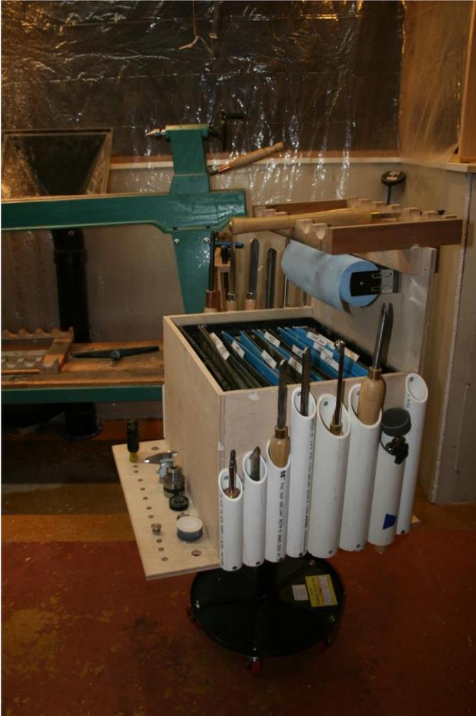
**This one works for me**, like other variations, plastic pipe holds gouges neatly, the box is a sandpaper organizer and the horizontal rack is a rest for tools currently in use and the whole thing rolls up next to the lathe. The base started life as an auto mechanic’s stool.
